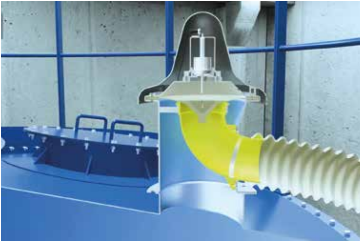
Silo top at the moment of overpressure relief through spring-loaded valve
